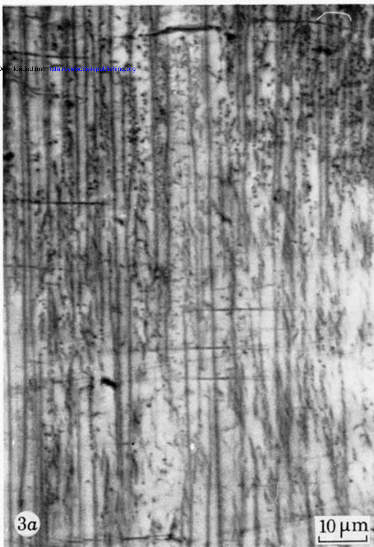
FIGURE 1. (110) slip band superimposed on the low stress dislocation substructure in a decorated olivine crystal from a basalt nodule (picture by Y. Gueguen).
