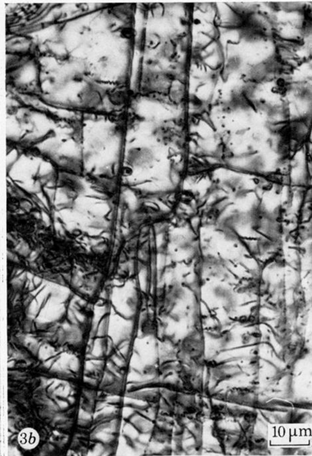
FIGURE 1. (110) slip band superimposed on the low stress dislocation substructure in a decorated olivine crystal from a basalt nodule (picture by Y. Gueguen).
